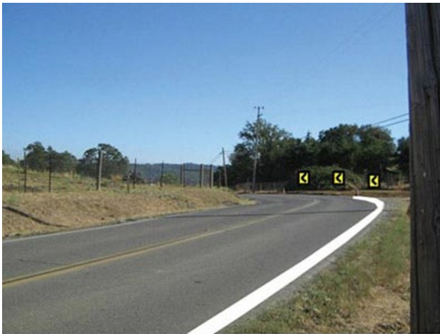
This edited photograph shows how safety could have been improved on McCourtney Road through low-cost countermeasures such as chevrons and better line delineation.
